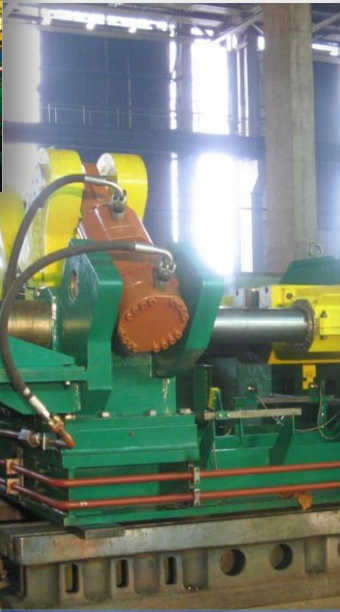
Swaging machine for OCTG tubes 139.7 - 339.7mm for JESCO Saudi Arabia, 2009
